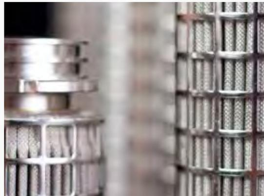
The cylindrical element design provides a sleeve of filter medium (protected and supported by woven meshes) around a support core. The pleated cartridge design uses a precision pleated pack (again comprising protection and support meshes either side of the filter medium) around a support core to provide nearly three times the effective filtration area of the cylindrical element.
