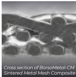
Magnification of BorsoMetal-CM Sintered Metal Mesh
